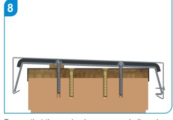
Ensure that the coping is secure and aligned on the front of the build. To further secure the coping, ARP recommends a secondary fixing with a self tapping screw be made on the internal edge through the coping into the fixing and jointing bracket.
