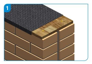
Before starting, it is important that there is a minimum of 18mm marine ply as well as a weatherproof membrane on top of the build.
