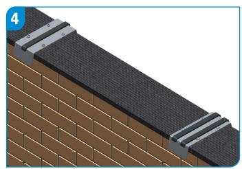
Jointing brackets will have 2 EPDM strips and fixing brackets have 1 strip. The fixing brackets should be spaced at a maximum of 1m apart and the jointing brackets directly under the 2 adjoining components. To ensure that there is correct alignment, it is recommended that the front edges of the brackets are level and in line.
