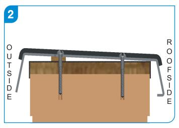
This guide is for sloping coping, which incorporates a standard 2° pitch, with the run-off directed towards the roof area and which reduces the liklihood of ponding on the coping surface.
