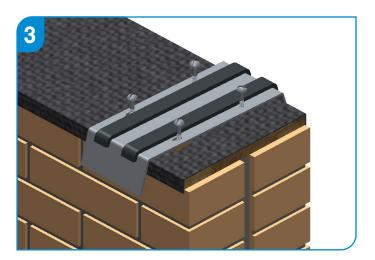
All coping components are supplied pre-drilled (for guidance only) and with EPDM sealing tape. The brackets should be secured to a depth of at least 50mm and should be suitable for the substrate. It is important that a secure fixing is made and consideration should be given where insulation has been installed on the outer face.
