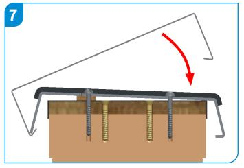
There will be some resistance as the coping compresses the EPDM strip, until the coping locates and clips over the internal edge.
