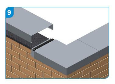
Installation should start at the corner, T-section or stopend/abutment and a line run along the front edge to ensure alignment. It is likely that at least one section of coping will need to be trimmed on site, so availability of the correct tools and touch-up paint is essential. To allow for thermal movement, it is recommended that 3-4mm is allowed as a gap between components.
