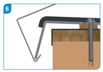
All coping and components are fitted by looping one edge over the external edge of the bracket and then pivoting the coping back the bracket towards the roofside.
